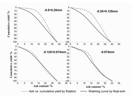
Fig. 5. Cumulative yield vs. ash of ground products separated by float-sink and progressive release flotation
