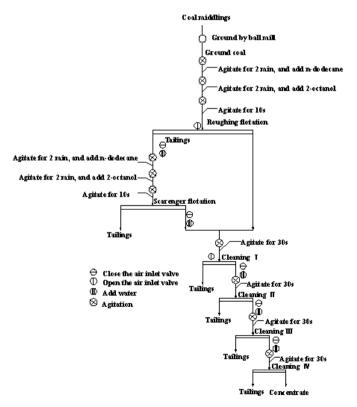
Fig. 1. Flow sheet of optimized progressive release flotation
